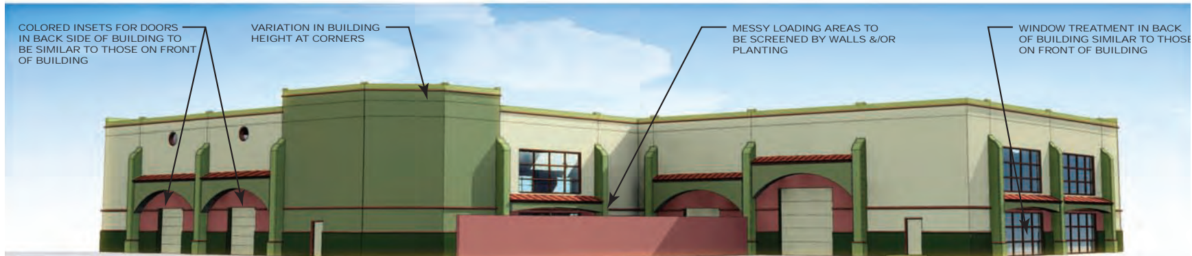
EXAMPLES OF INDUSTRIAL BUILDINGS REAR ELEVATION OF TWO STORY - COLOR ALT. #4
