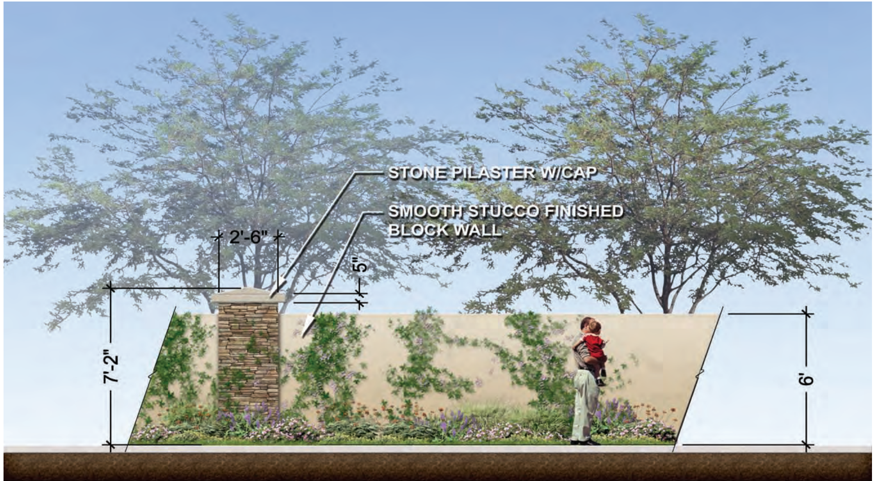
Exhibit 99 | Stucco Finished Wall With Stone Pilasters
